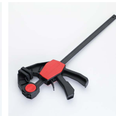
PE0830 Value Bar Clamp Size: 12"/300 Material: nylon clip block +PP guide +A3 steel surface electrophoresis black Color customized
