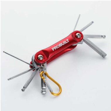
PE0344 8Pc Folding Ball End Hex Key Set Size: 2mm, 2.5mm, 3mm, 4mm, 5mm, 6mm, 8mm, 10mm Material: 40Cr Hex Key, Aluminum Handle Finish: Matt Chromep Plated Customized Handle Color
