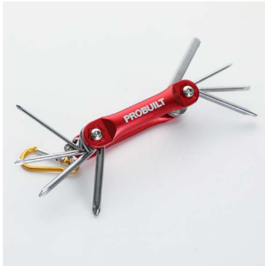
PE0343 8Pc Folding Hex Key Set Size: +, PH0, PH1,PH2,PH3, -3.0mm,4.0mm,5.0m,6.0mm Material: 40Cr Hex Key, Aluminum Handle Finish: Matt Chromep Plated Customized Handle Color
